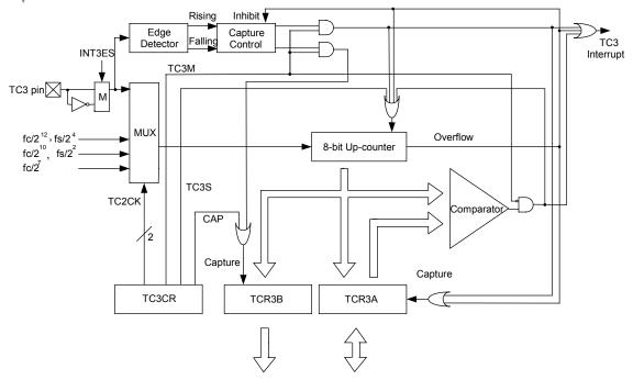
Fig. 23. Configuration of Timer/Counter3
